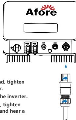
1. Connect AC terminals and waterproof head, tighten the cap, make sure they clip closely together.
