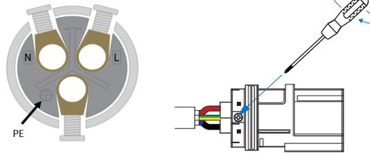
Connect AC line, Live line (L), Neutral line (N) and Ground Wire (PE) according to polarity.
