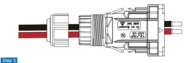
Insert the wire harness into the terminals according to "+" and "-" polarity, make the insulated terminals parallel with the terminals , the crimping screw torque is 2.0±0.1N.m
