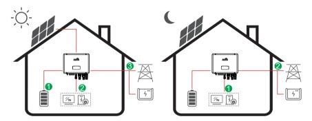
Energy flow: PV → Battery → Load→ Grid
