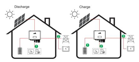
**Energy flow:** Discharge: Battery and  $PV \rightarrow Load \rightarrow Grid$
