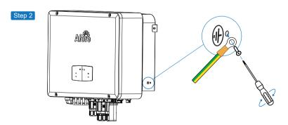
Fix the grounding screw to the grounding connection of the machine housing.
