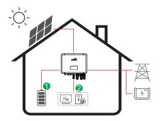
Energy flow: Grid power > P\_Back : Battery and PV  $\rightarrow$  Load
