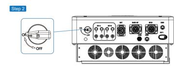
Turn on the DC switch and AC circuit breaker, and wait until the LED indicator on the monitoring module flashes, indicating that the monitoring module is successfully connected.
