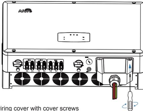
Fix the AC wiring cover with cover screws
