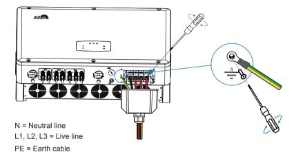
Unscrew the row of screws, insert the wire harness into the N, L1, L2, L3 caps one by one, and tighten the screws.
