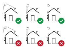
• The inverter should be installed vertically on the wall, or lean back on plane with a limited tilted angle. Please refer to below picture.
