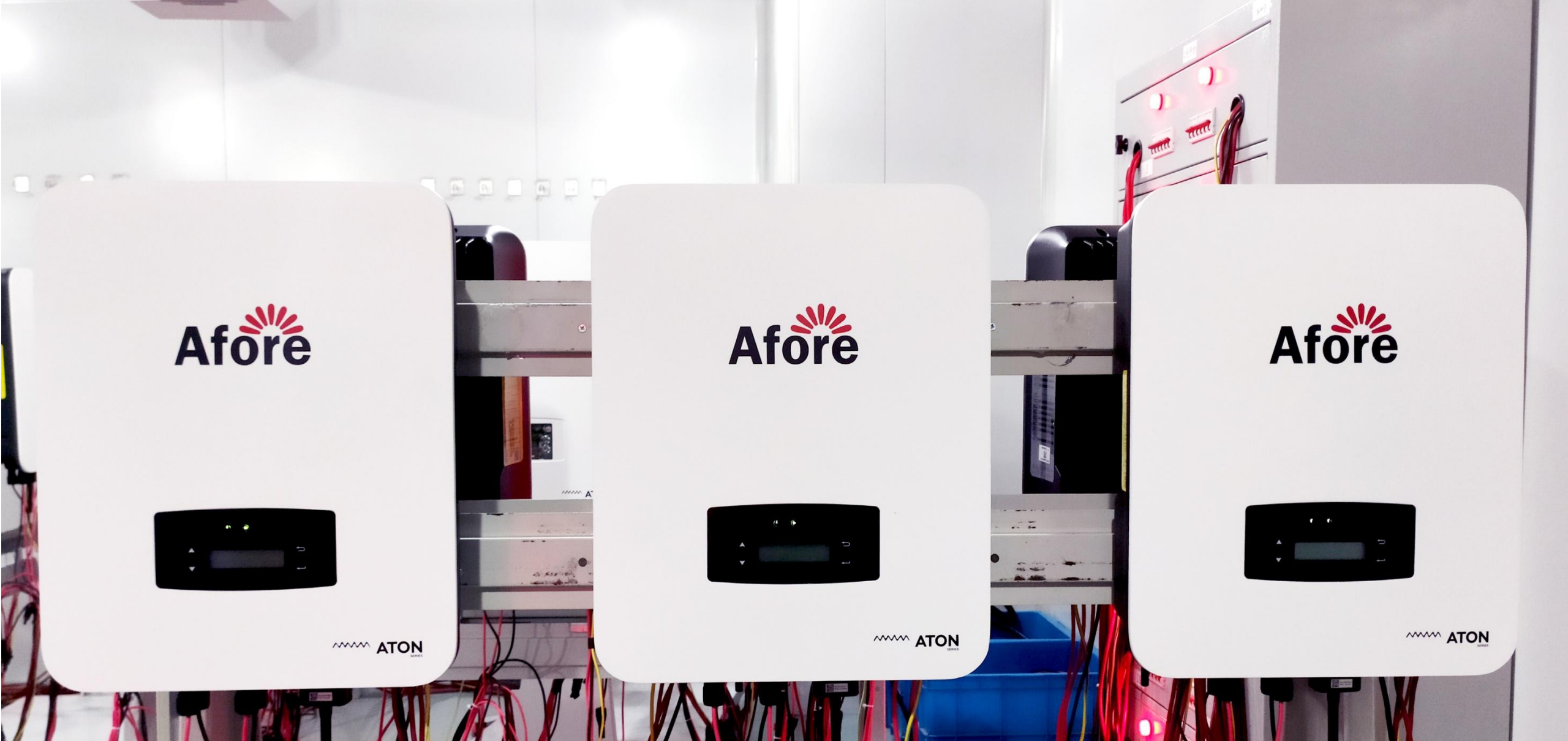
Inside the high temperature chamber, every inverter goes through up to 8Hrs Aging Test without power degrade.
