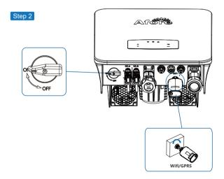
Turn on the DC switch and AC circuit breaker, and wait until the LED indicator on the monitoring module flashes, indicating that the monitoring module is successfully connected.
