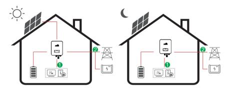
**Energy flow:** Battery and  $PV \rightarrow Load \rightarrow Grid$
