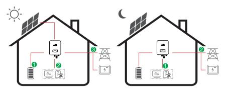
Energy flow: PV → Battery → Load→ Grid
